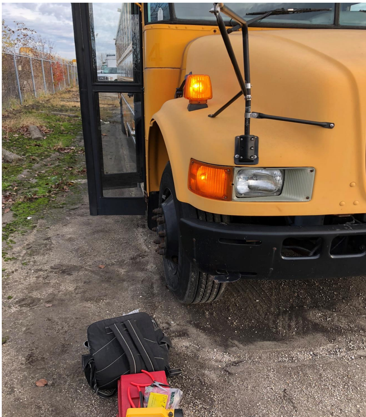
Turn indicator works after replacement. Wire harness was tugged and wiggled with no adverse affect to turn indicator operation.
